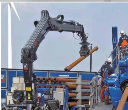
Drill pipe crane with remote control
