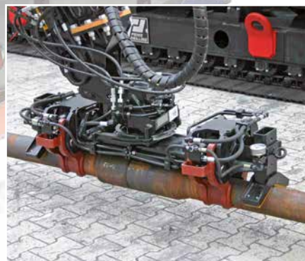
Three dimensional drill pipe gripper, rotating and pivoting
