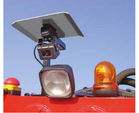
Camera and lights for power rotary head and breakout system
