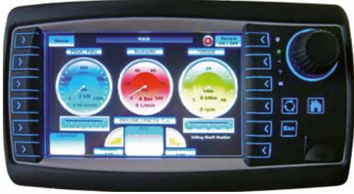
Drill data monitoring system records all drill data parameters
