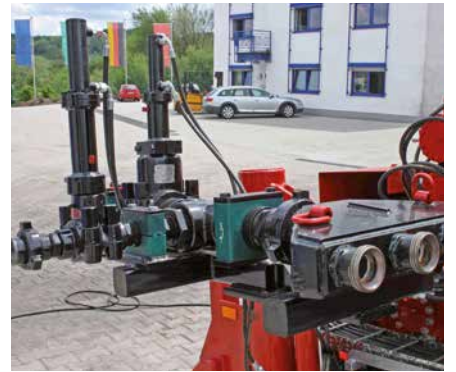
Bentonite supply, hydraulically lockable with by-pass
