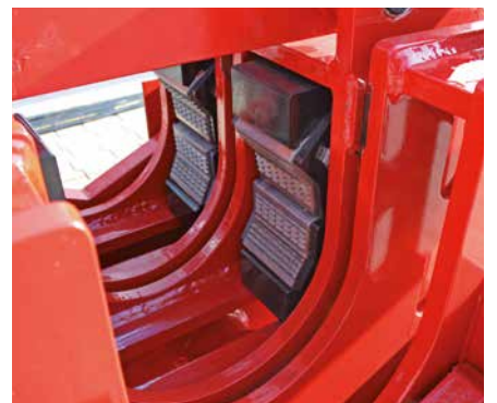
Breakout system with easy replaceable and self-centering clamping jaws
