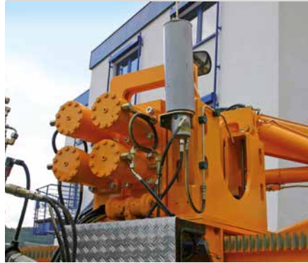
Automatic drill pipe lubrication system
