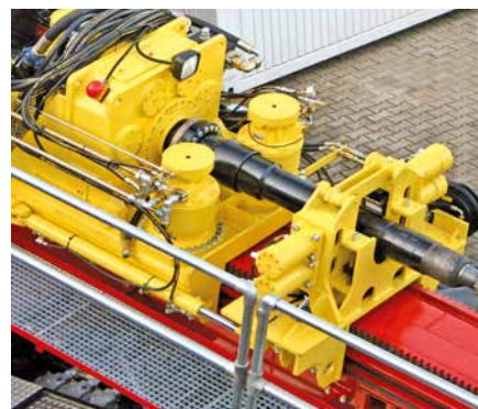
Breakout system at the power rotary head
