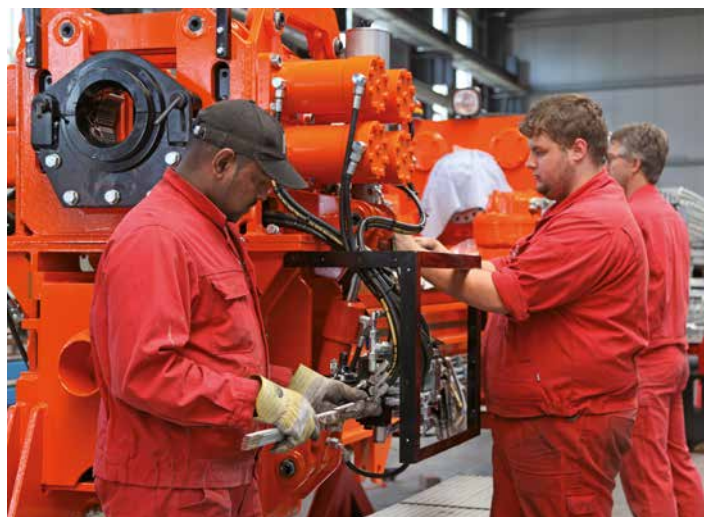
Final installation of a drill mast
