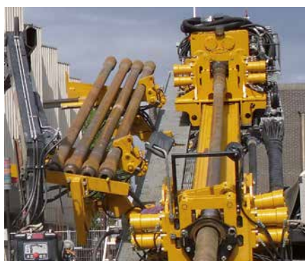
Drill pipe supply for 5 drill pipes
