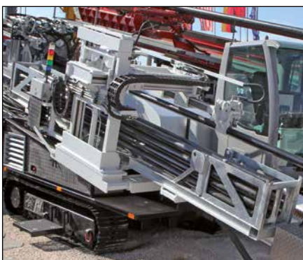
Fully automatic drill pipe magazine for 72 m drill pipes
