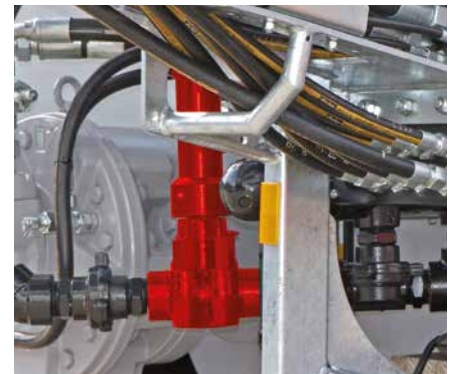
Bentonite supply, hydraulically lockable with by-pass
