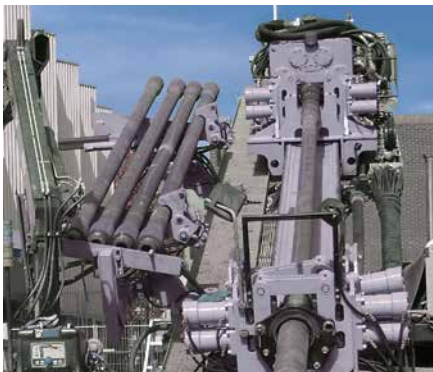
Semi-automatic drill pipe supply for 5 m drill pipes
