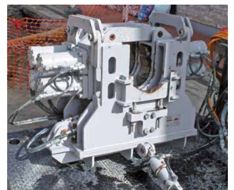
Pipe-site breakout system with adjustable exit angle 6° - 22°
