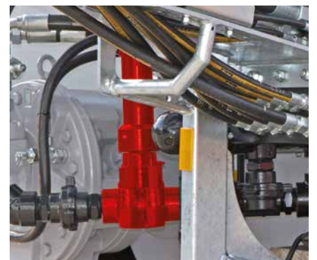
Bentonite supply, hydraulically lockable with by-pass
