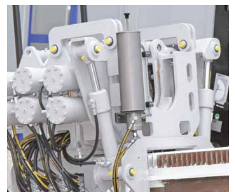
Automatic drill pipe lubrication system
