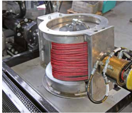
Cable reel with hydraulic motor and electric swivel guide
