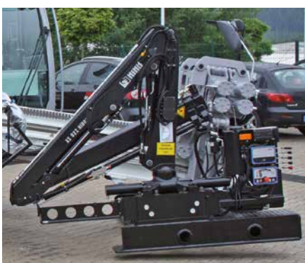
Drill pipe crane with remote control
