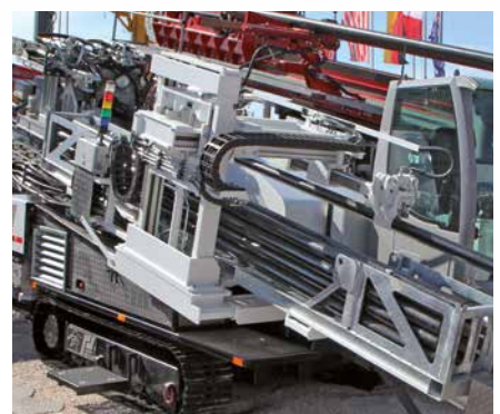
Fully automatic drill pipe magazine for 12 drill pipes
