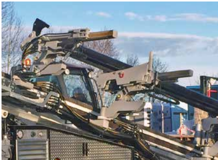
Semi-automatic drill pipe supply for 5 drill pipes
